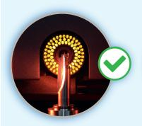
Use non-contact type equipments for presetting and measuring T.I.R
