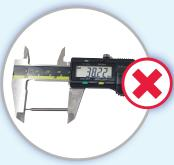
Do not directly load the Tool in Vernier for measurement
