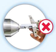
Avoid contact type method. By this tool can be damaged before usage
