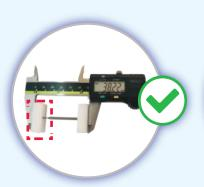
Use POM / Acrylic sheet to avoid damage before measurement
